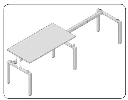
With the assistance of at least 1 other person, gently lower the top into position over the frame, resting it on the spacers and the beam. Once the top is in position, line up the outside leg more accurately with the end of the desk top taking care to avoid knocking the spacers out of position.
