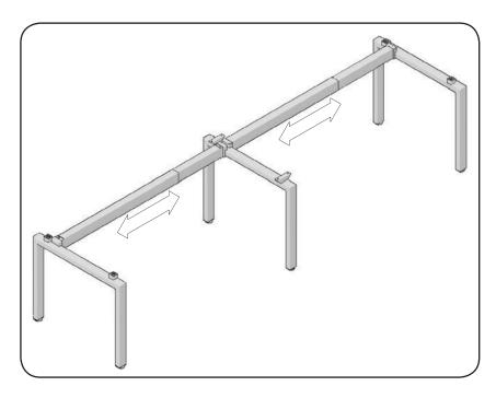
Repeat steps 2 to 4 with the remaining legs and beams. If your bench consists of multiple desks just keep adding the sections one by one. It is advisable to build up the frame in this way so it is in the desired position for the finished bench as large benches can be difficult to move.
