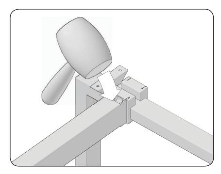
Using the mallet secure the end of the beam fully into the intermediate leg by tapping at the end so as not to damage the top of the beam.
