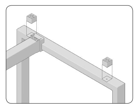
Take the four plastic spacers supplied with the legs (two with each leg) and place one over each of the holes in the leg frame, aligning the holes in each spacer roughly with the corresponding hole in the leg. The spacer has a small lip which should fit over the radius on the edge of the leg.
