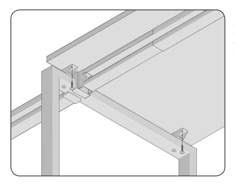
Using two 15mm bolts secure the top to the intermediate leg by placing them through the holes in the wedge shaped spacers and into the underside of the desk top. Fully tighten these bolts.
