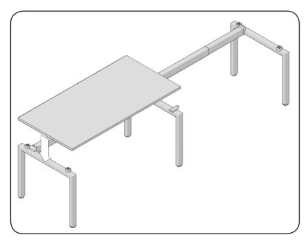
With the assistance of at least 1 other person, gently lower the top into position over the frame, resting it on the spacers and the beam. Once the top is in position, line up the outside leg more accurately with the end of the desk top taking care to avoid knocking the spacers out of position.
