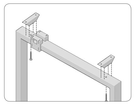
To start with assemble the intermediate leg in its entirety; take the leg along with the wedge shaped spacers and two 55mm bolts. Insert the bolts up though the holes in the leg frame and into the threaded holes on the underside of the spacers. Tighten them so they are secure but do not over-tighten. You should not have to use excessive force to tighten the bolts adequately.
