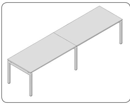
Repeat the previous 5 steps using the remaining leg frame, or if your bench consists of multiple tops, keep working along its length in this way ensuring all fixing bolts are securely tightened.
