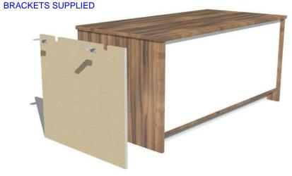
OFFER UP THE INFILL PANEL TO THE END PANEL OF THE DESK, ENSURING AN EVEN BREAK (2mm) FRONT AND BACK. USE THIS INFILL PANEL AS A JIG TO POSITION THE BRACKETS ON THE DESK.
