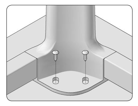
Place the black 'mush head' screws through the holes in each leg and screw them into the underside of the top using the 4mm Allen key. Continue turning until the fully inserted but avoid over-tightening.
