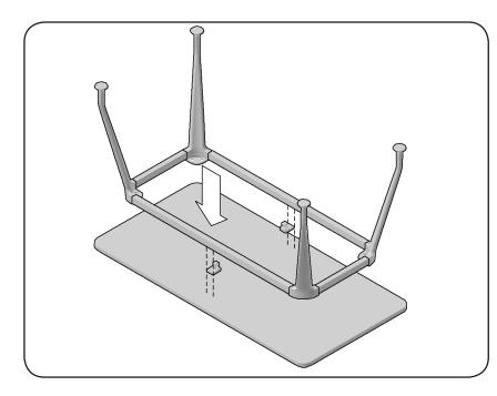
Lay the top on the floor, underside facing up (pilot holes facing up). Place the frame on top of it as shown and align the two oval shaped holes in each leg with the pilot holes in the top. Place the spacer hooks, one under each of the long beams, with the hooks facing towards the centre of the desk and the beam sitting in the shallow recess in the block.
