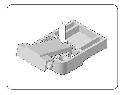
Take all the spacer hook components (grey plastic) out of their packaging. Take one of the rectangular blocks and one of the hooks. With the 'Verco' and '100-DNASH' text on the inside of the moulding facing up, insert the hook in to the central hole as shown left.
