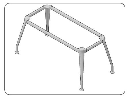
In the same way as the short beam place and fix the long beams in between the two structures. Place both beams before securing them in place as once one is in place the structure will be locked in place.
