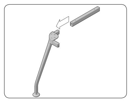
Take one of the corner legs and one of the shorter rails (if you have a DD0808 or DD 1616 all rails will be the same length so start with any of them). With the holes in the rail facing upwards, insert either end of the rail onto one of the metal lugs at the top of the leg. If the rail will not slide on easily ensure that the bolts in the lug are fully retracted by turning them clockwise with the Allen key.
