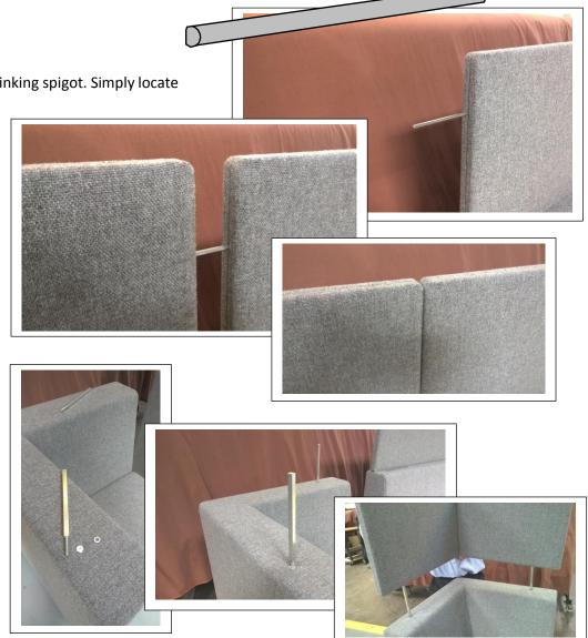
**CORNER** and **TEE** screens Remove the transit screws and screw in the spigot making sure that the washer supplied is fitted, to protect the fabric. ... then locate and drop the screen onto the spigots and link, as above.
